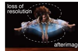
3D Noise Reduction Alone Afterimage and some loss of resolution is seen
