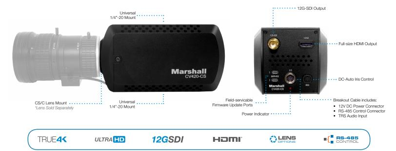
The **Marshall CV420-CS** is a true 4K camera built around a 12.4-Megapixel, 1/1.7-inch sensor delivering ultra-crisp, clear true 4K resolution in 4096x2160p at 60fps. CV420-CS contains a single 12G (BNC) and a simultaneous HDMI 2.0 output covering a variety of 4K/UHD/HD applications. Flexible CS/C lens mount format offers a wide range of lens options with DC Auto-Iris plug-in capability.
