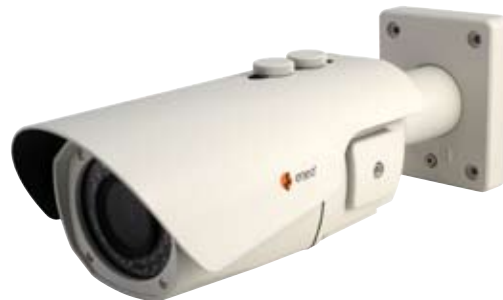
Art.: 200264 Caméra 1/4", jour&nuit, WDR, BLC, 12x, 3,8-45,6mm, 650ITV, 12V/24V, illumination IR, IP68
