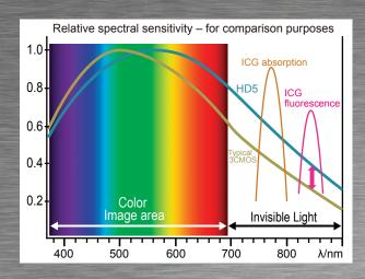
Incorporating Toshiba's innovative three-chip technology, the IK-HD5 provides approximately 3dB-increased sensitivity in the near-infrared spectrum through 700-870 nm. When equipped with the appropriate optics and filters, the IK-HD5 can be used for both visible light and near IR imaging applications such as indocyanine green (ICG) and other fluorescing agents
